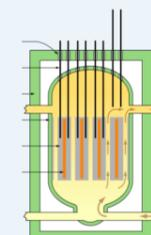
**5.10 Describe how thermal (heat) energy from the chain reaction is converted into electrical energy in a nuclear power station**
